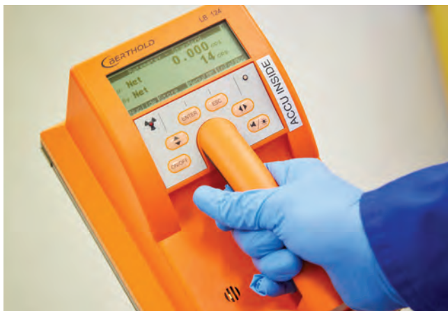
A contamination monitor is used to make sure surfaces, samples and people aren't contaminated when we work with unsealed radioactive sources.
