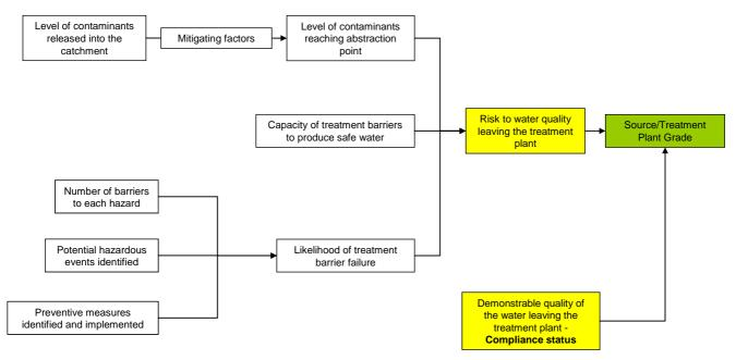
Fig. 3.1 Conceptual basis for the source-treatment plant grading - Model 1
