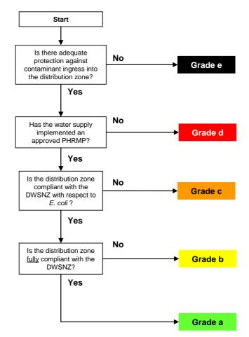
Fig. 5.2Derivation of distribution zone grades – Model 3
